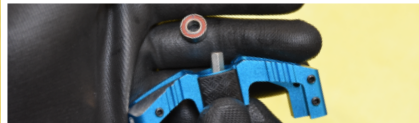
8. PUSH OUT THE CARTRIDGE BEARING USING THE LONG HANDLE 6MM HEX WRENCH.
