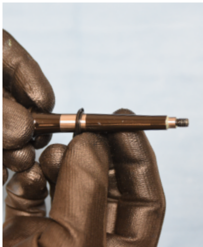
12. INSTALL THE OUTER SPINDLE SEAL FIRST, ROUNDED EDGE FACING AWAY FROM SMALL END OF THE SPINDLE. INSTALL THE INNER SEAL (DOUBLE-LIP SEAL) WITH THE POINTED END FACING TOWARD THE LARGE END OF THE SPINDLE.
