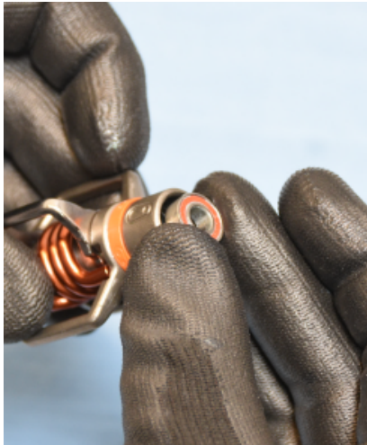
11. INSTALL CARTRIDGE BEARING INTO OUTER BODY.
