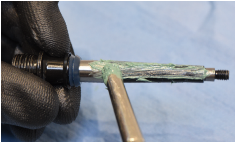
13. LIGHTLY COAT THE SPINDLE WITH GREASE. (DO NOT GREASE THE THREADS AT THE SPINDLE END)
