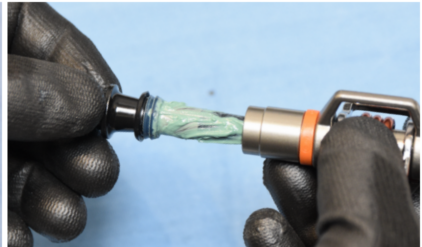
14. INSERT THE SPINDLE INTO PEDAL AND THROUGH CARTRIDGE BEARING.
